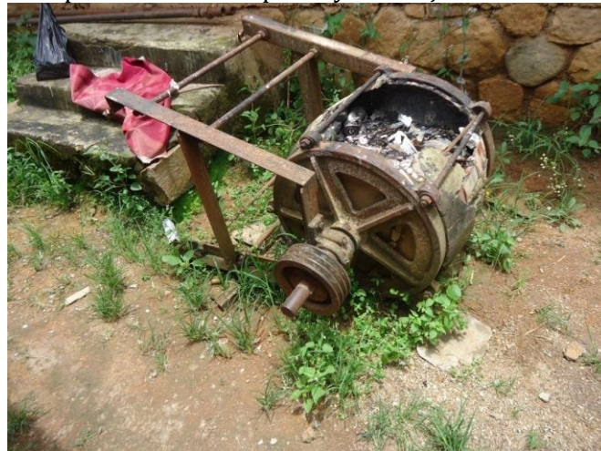
Figure 6: After the fire accident the Ball Mill now serves as a dustbin (Photo by Gukas 2016).
