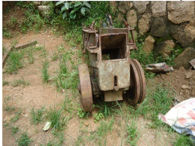
Figure 7: The Pug Mill after the fire accident at the centre. (Photo by Gukas 2016)
