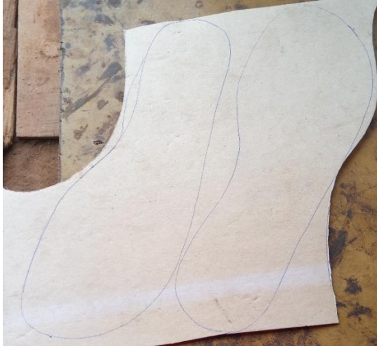
Plate 3: marking out the shape of the feet on a fibre. Source: C. Chudi-Duru (2017)
