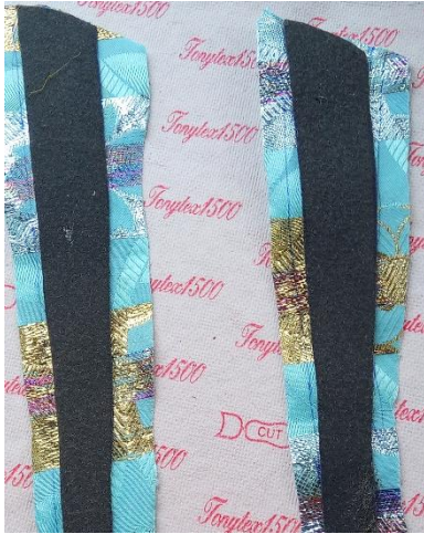
Plate 5: sticking the upper to the cut out fibre for reinforcement. Source: C. Chudi-Duru (2017)
