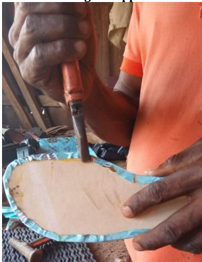
Plate 6: making sure that the fabric is well stuck to the innersole. Source: C. Chudi-Duru (2017)
