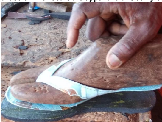
Plate 7: temporary fixing of the upper to the last. Source: C. Chudi-Duru (2017)
