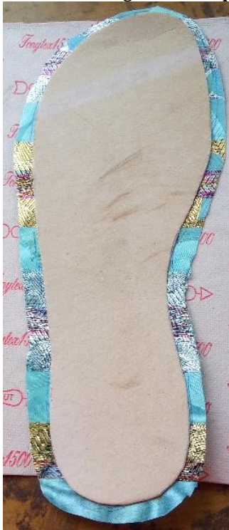
Plate 4: sticking the cut out shape with evo-stick to the fabric cut. Source: C. Chudi-Duru (2017)
