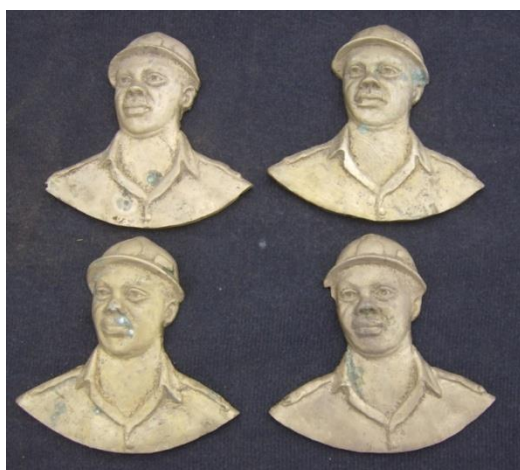
Fig. 7: 'Oil Worker' brass casts meant for award plaques design cast at Igun street. This portrays mass-production possibilities of metal casting. Location: Metal Design Unit, Department of Fine and Applied arts, University of Benin. Photograph by Kingsley Emeriewen, 2016.
