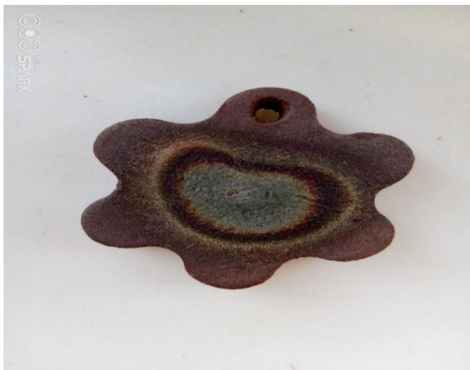
Plate X: CCCSA fired in a reduced atmosphere to 1100 0 C Source: Research Photograph, Sheikh (2019)
