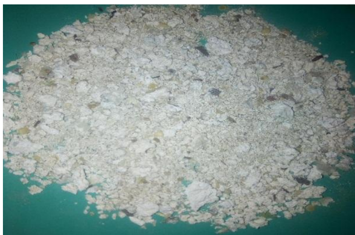
Plate VII: Colour Changes to Grey white when exposed to the atmosphere for 24hrs
