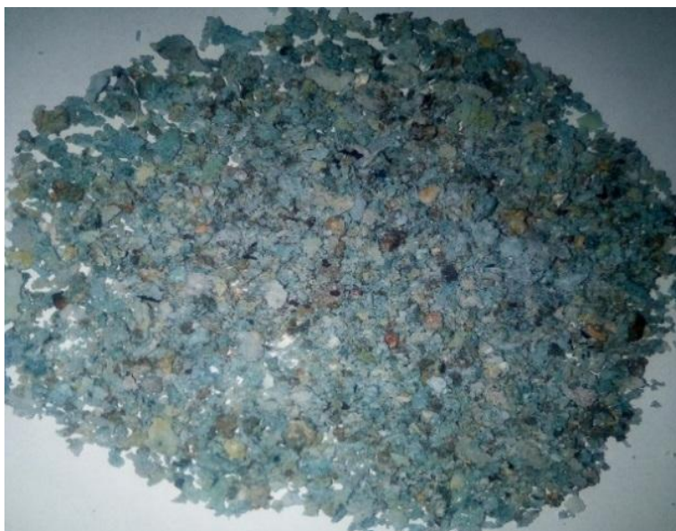
Plate VI: CCCSA fired to 800^{\circ}C at reduction atmosphere
