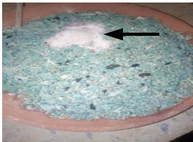
Plate IX: Inset: the colour of the rice husk did not change when fired to 930°C
