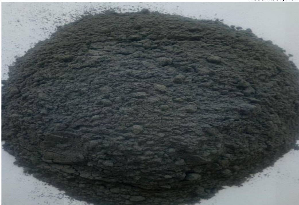
Plate V: CCCSA ready for sieving---Powdered through 40-mesh sieve Source: Research Photograph, Sheikh (2019)
