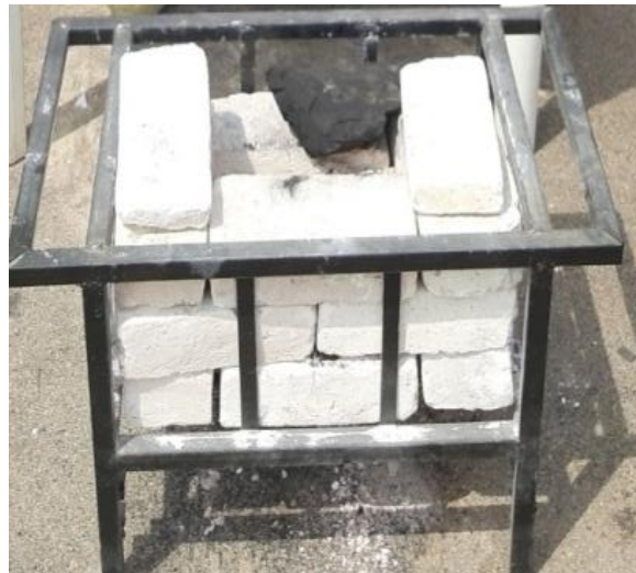
Plate VI a: Yoyang Refractory Brick Stove in Fabricated Metal Case
