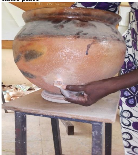
Plate III, Fixing of the Pipe Head that Filtered Water Can Pass through
