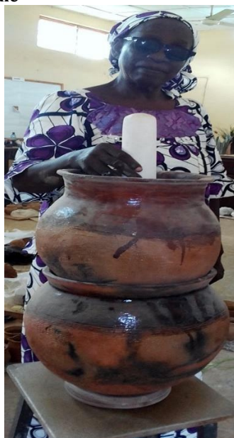
Plate II. Fixing of Water Filter Candle into Pots Which Heterogeneous Water Mixture Separation by Filtration takes place
