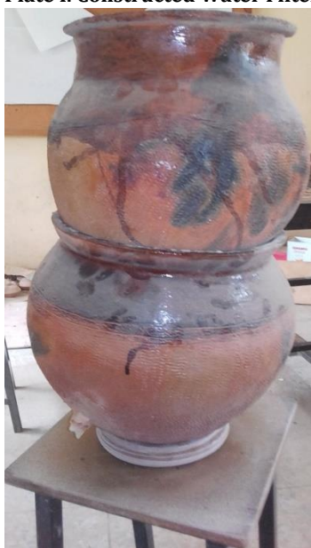
Plate II. Fixing of Water Filter Candle into Pots Which Heterogeneous Water Mixture Separation by Filtration takes place
