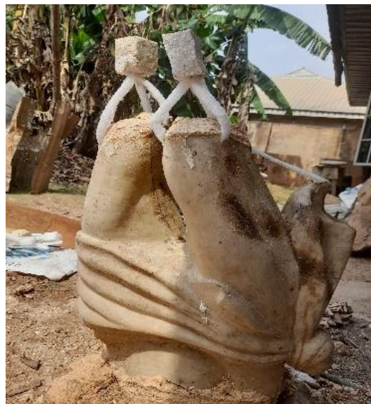
Plate 4: Sprue-Wax Work with Core. Source: NJK Studio University of Benin, 2021.
