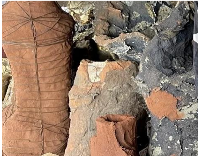
Plate 2: Invested Moulds in Traditional Laterite Method. Source: https://www.oluwalanu.com/post/bronze-casting-in-benin-a-unique-retrieved , June 11, 2025.
