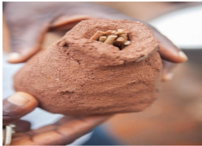
Plate 3: The Traditionally Invested Laterite Moulds. Source: https://www.facebook.com/photo.php?fbid=670962282962547&id=155689984489782&set=a Retrieved, 9/6/2025
