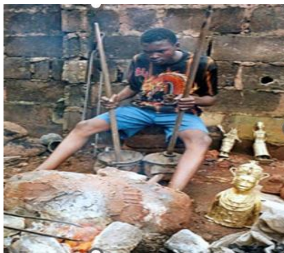
Plate 7: The Traditional Hand Bellow System. Source:
