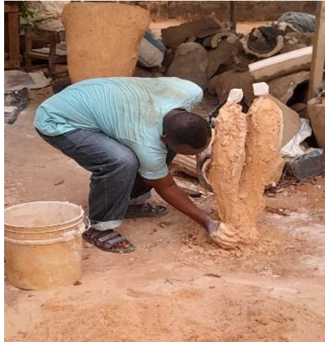
Plate 5: The Researcher Investing with Plaster. Source: NJK Studio University of Benin, 2021.
