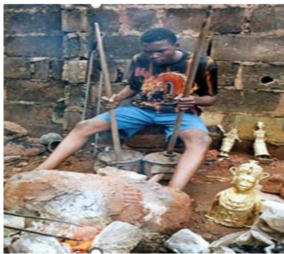
Plate 7: The Traditional Hand Bellow System. Source:
