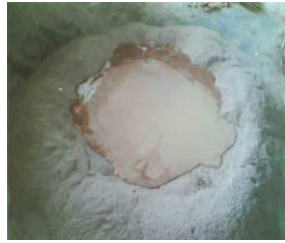
Fig. 3 mixing of watery clay and grog
