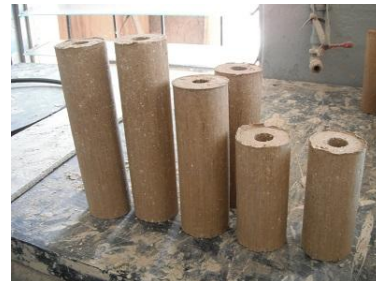
Fig. 8 extruded props positioned for drying
