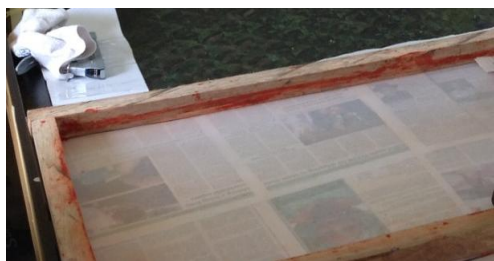
Plate 7: Stretched Printing Frame
