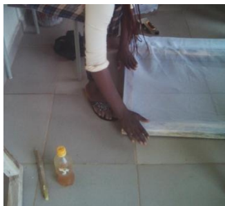
Plate 6: Stretching of Printing Screen
