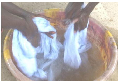
Plate 8: De-sizing of Fabric
